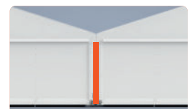
Connecting gutter between aluminum halls
