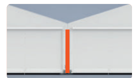
Connecting gutter between alu halls
