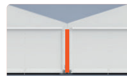
Connecting gutter between alu halls
